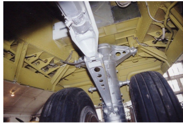
2002-03 Aft Main Gear
