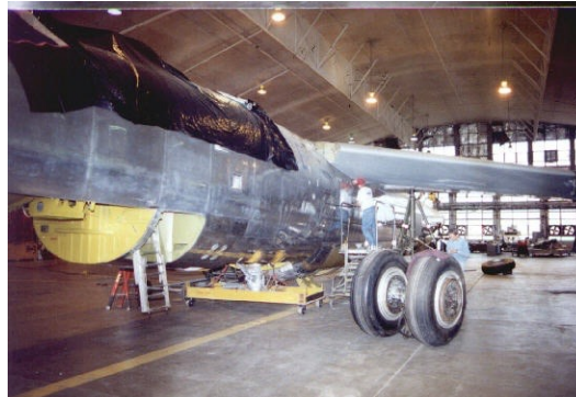
2002-03 Install Wing Panels
