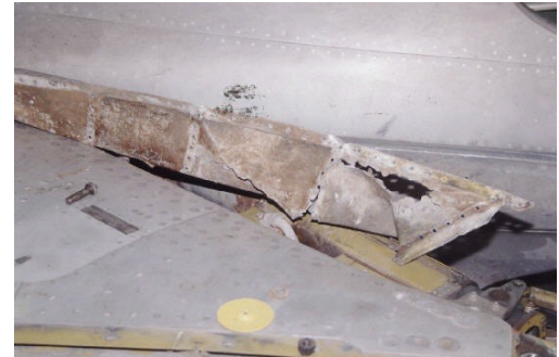
2002-03 Engine Mount Corrosion
