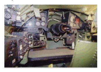
Navigator's station in the nose. Restoration could not find a ten-inch radarscope, so they likely got this one from a tanker.
